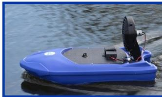
The TORMADA® is an unmanned lightweight product application boat that enables ponds and dock areas to be treated for weeds and algae without launching a manned boat by
